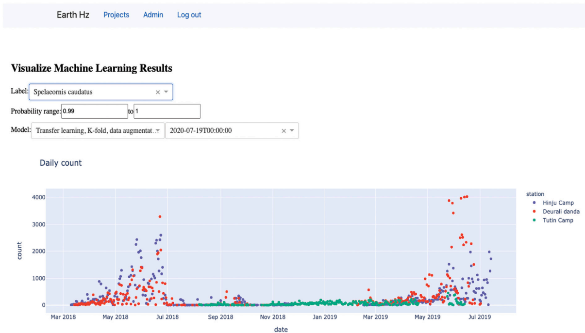
Fig. 4. Web interface that can visualize the number of detected calls in multiple monitoring stations over time for certain targeted species. The interface allows the users to choose different probability ranges from model predictions.
